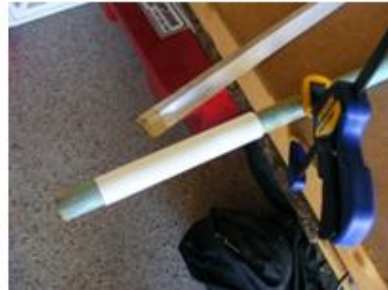
Figure 2. Body tube splitting jig
