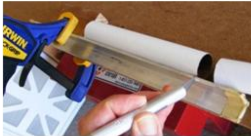
Figure 1. Body tube cutting jig
