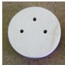
Figure 4. Bulkhead hole layout
